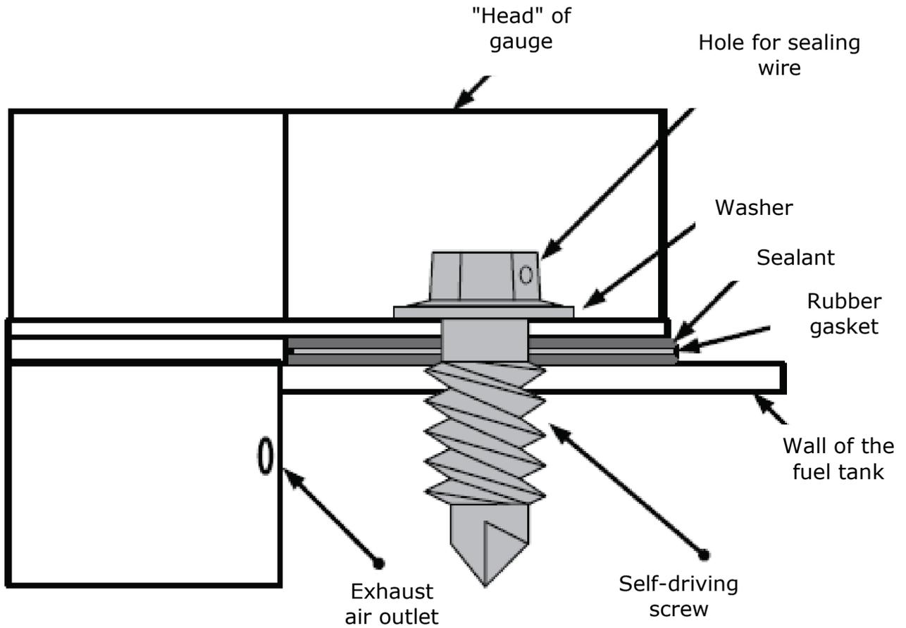
Fixing with self-driving screw
