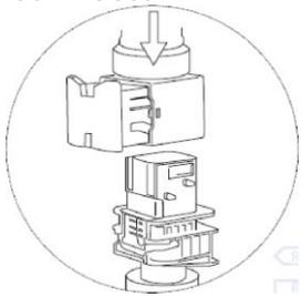
Keep the connector pressed and close the slide
