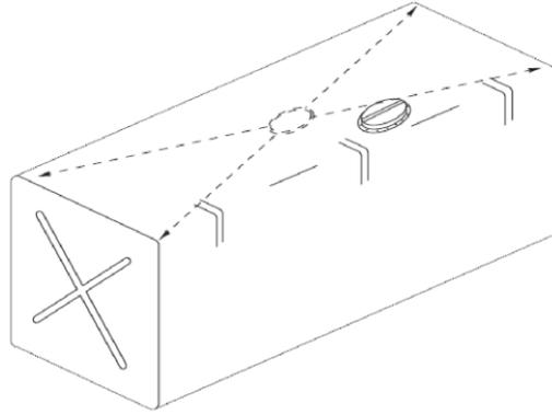
If the tank is specially shaped and has two upper levels or overflow holes, we recommend that you install 2 fuel gauges to eliminate the deadzones of measuring.
