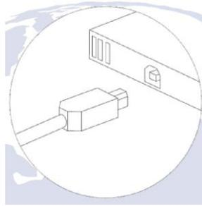
Release the slide by clicking on the socket connector
