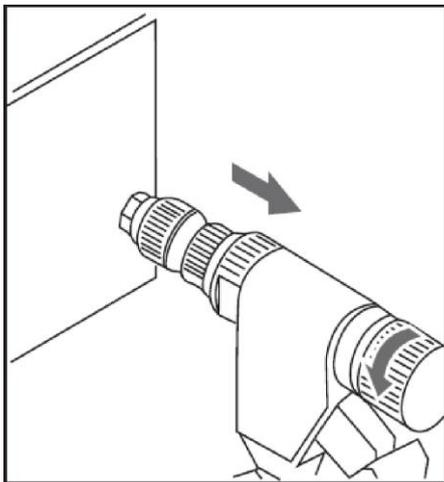
If the rivet is mounted incorrectly, is loose or it is difficult to screw the fixing screw, drill out the rivet tool and adjust the lock nut of the tool and the front sleeve according to the scheme provided below.
