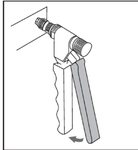
Remove the core of the riveter from the mounted rivet.
