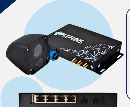
Bitrek's NVR is an automotive network recorder with an external GSM and GPS module, 2 bands of WiFi, and Bluetooth onboard. It supports up to 8 IP cameras, it has 128 MB VPN protection, up to 2TB storage, and Bitrek's CAN interface for attaching external sensors and modules.
