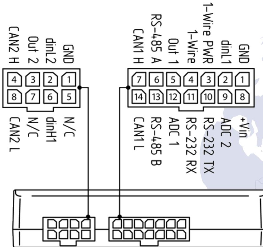
Figure 2. Pin assignments
