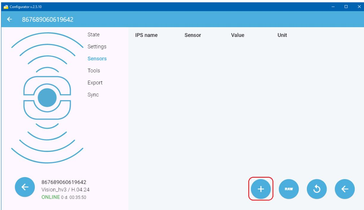
Figure 26. Adding a CAN sensor in manual mode
