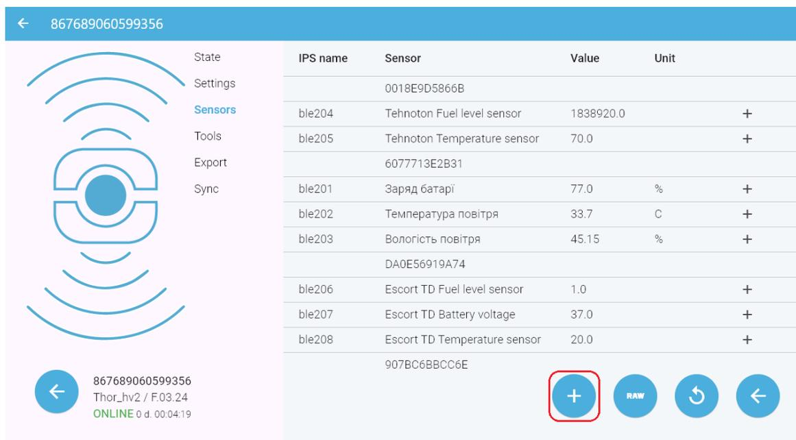
Figure 32. Manual adding of BLE sensor
