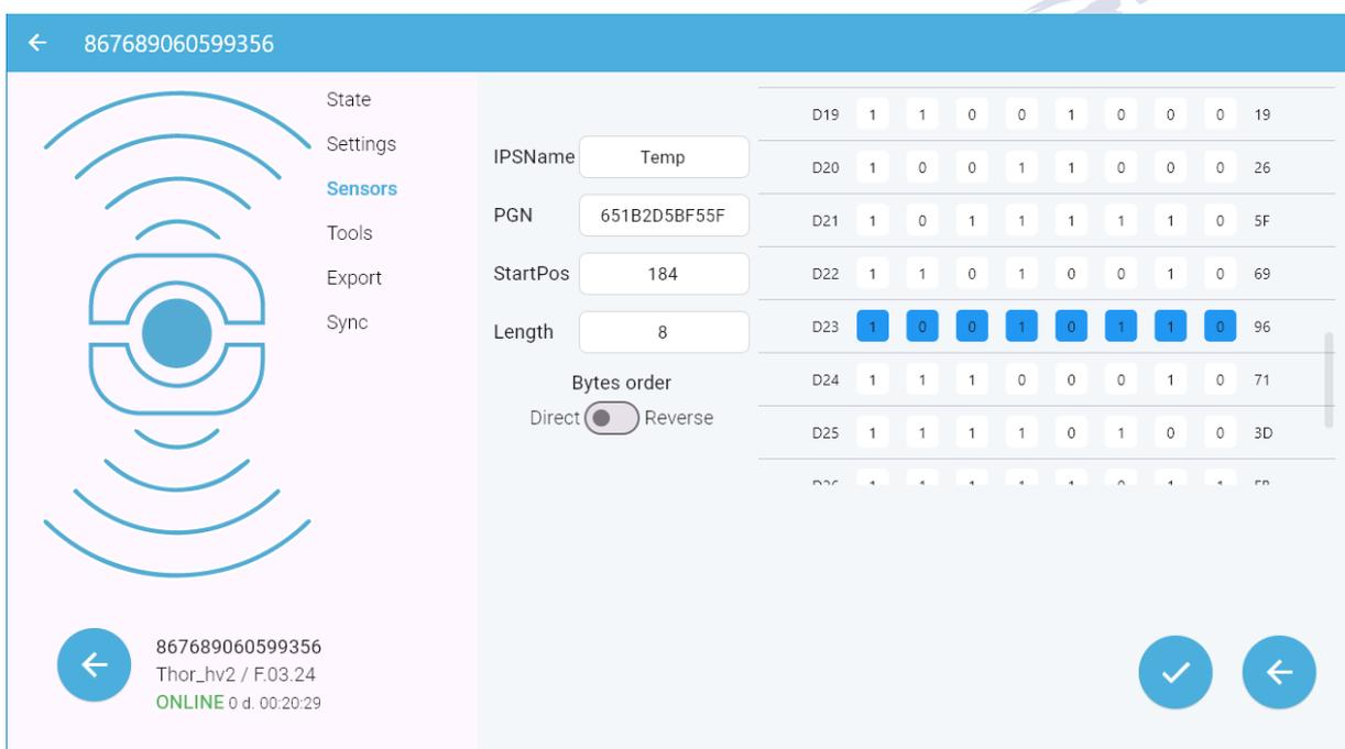
Figure 35. Sensor addition with direct data byte order (little-endian)
