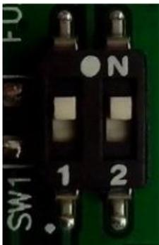
Figure 20. CAN and RS-485 bus terminating resistor switch
